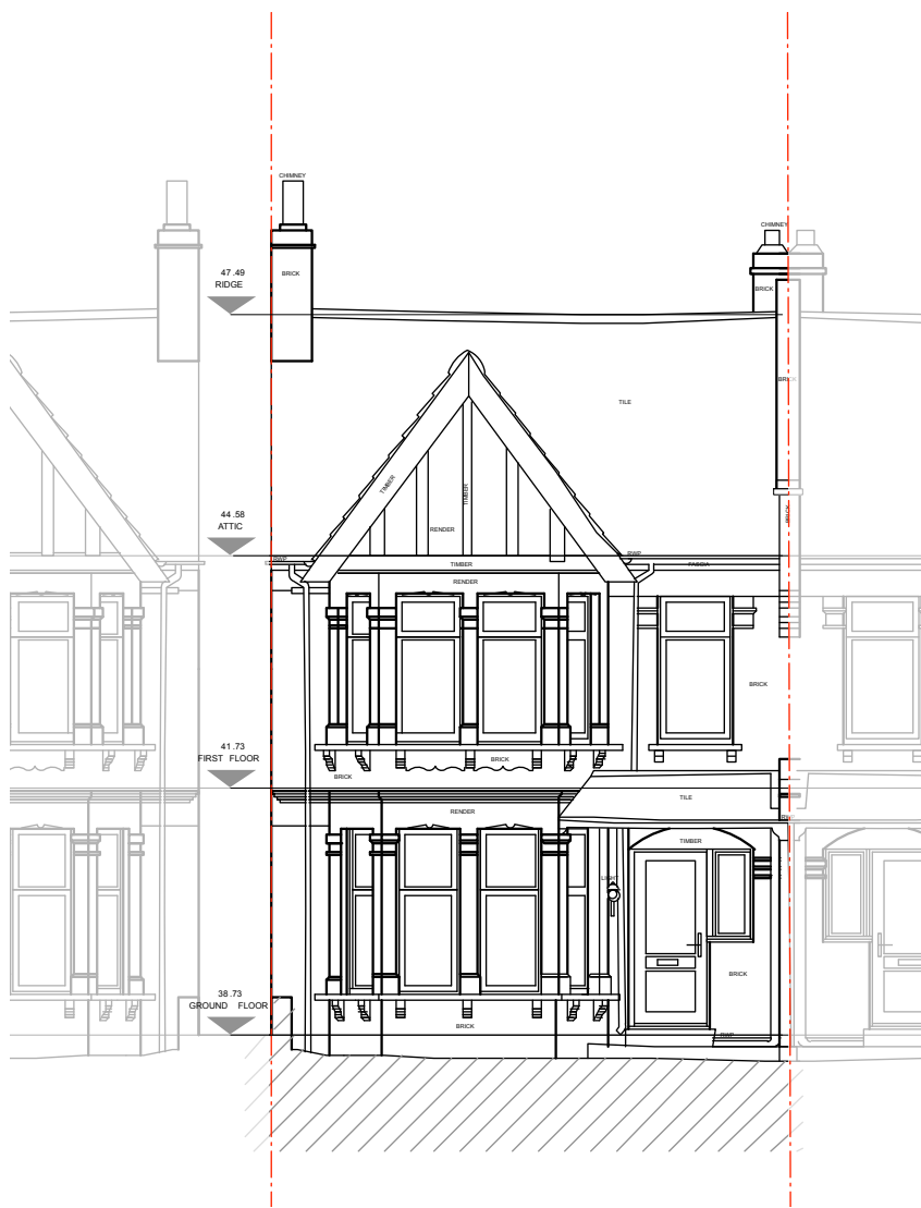
2. EXISTING FRONT ELEVATION
